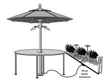
**Connect to 12V Landscape Lighting System** (Recommended Method) Compatible with both LED and Halogen
