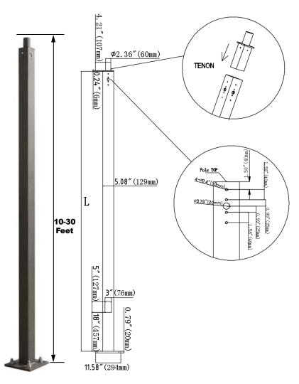
The LS Series Straight Square Steel poles are built from high strength steel tube and are available side drilled for arm mounted area lighting luminaires or with tenon mounts for flood and post top luminaires. Typical area lighting applications include retail centers, industrial parks, schools and universities, public transit and airports, office buildings and medical facilities. Mounting heights of 10 to 30 feet can be used based on selected luminaire application.
