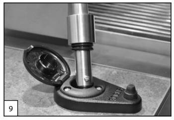
(9) Insert Quick Connect BBQ fixture into base with set screw facing towards front of counter. Press fixture firmly into place. Turn on power and check for proper operation.
