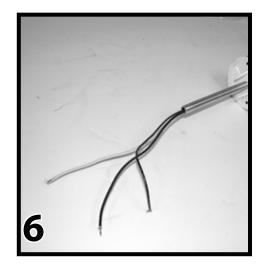
Attach Power Cord to terminals on plug.
