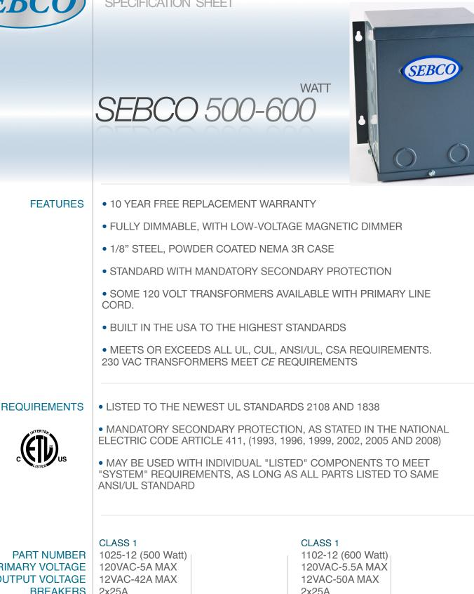
PART NUMBER PRIMARY VOLTAGE OUTPUT VOLTAGE BREAKERS FREQUENCY DIMENSIONS WEIGHT
