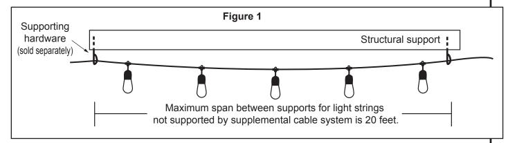
3. For spans exceeding 20 feet, use properly rated cable support system and cable ties (neither are provided with the light string) and follow local codes for suspended structures and loads. See www.americanlighting.com for steel cable support systems, if needed.
