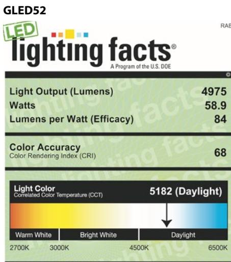
All results are according to IESNA LM-79-2008: Approved Method for the Electrical and Photometric Testing of Solid-State Lighting. The U.S. Department of Energy (DOE) verifies product test data and results.
